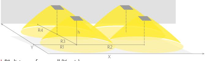
R1 distance from wall (X axis) R2 installation distance between lights (X axis) R3 installation distance between lights (Y axis) R4 distance from wall (Y axis) twsc292wac
