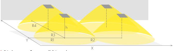
R1 distance from wall (X axis) R2 installation distance between lights (X axis) R3 installation distance between lights (Y axis) R4 distance from wall (Y axis) TWT3252WA
