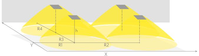
R1 distance from wall (X axis) R2 installation distance between lights (X axis) R3 installation distance between lights (Y axis)
