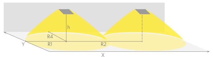
R1 distance from wall (X axis) R2 installation distance between lights (X axis) R4 distance from wall (Y axis) Y4252WM
