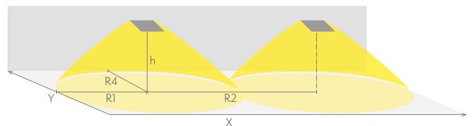
R1 distance from wall (X axis) R2 installation distance between lights (X axis) R4 distance from wall (Y axis) YB152WA120
